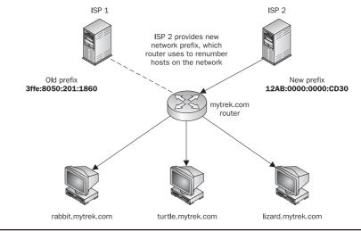
FIGURE 35-2 Router renumbering with IPv6 autoconfiguration
