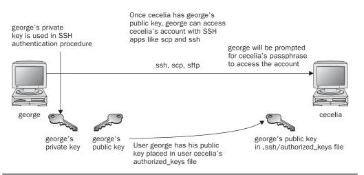
FIGURE 19-1 SSH setup and access
