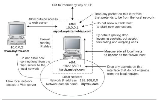
FIGURE 20-2 Firewall rules applied to a local network example
