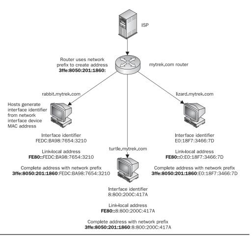
FIGURE 35-1 Stateless IPv6 address autoconfiguration
