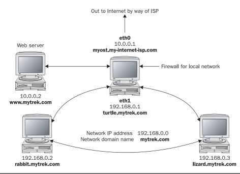
FIGURE 20-1 A network with a firewall
